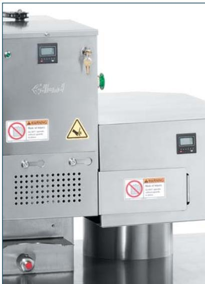
Two lockable, programmable counters for accurate lid-to-can verification
